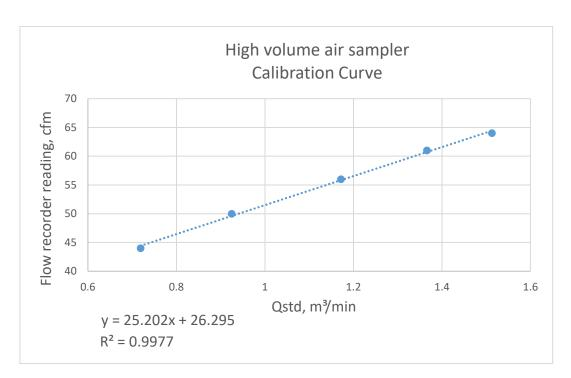
Note : The coefficient of determination (R<sup>2</sup>) of the calibration curve greater than 0.99 after a 5-point calibration, the high volume air sampler complies with the specified requirements and deemed acceptable for use.
